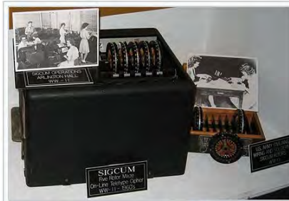
Rotor machines, like this SIGCUM , were an early source of compromising TEMPEST effects
