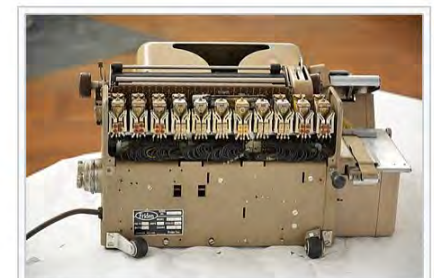
Relay logic, such as in this Flexowriter was another major early source of TEMPEST radiation.
